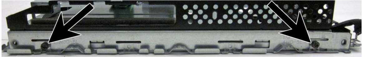
Figure 6-85 Display panel screw locations – 6300 models – LG or AUO panel
